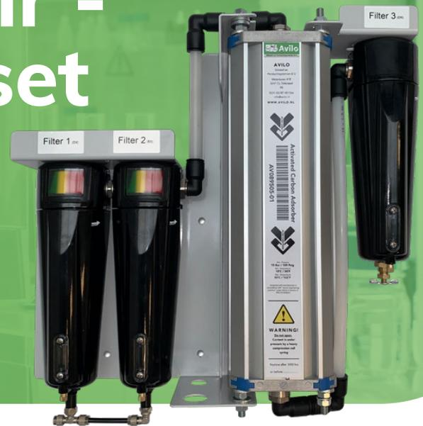
However, it is an excellent general filtration set-up for other applications as well. The set consists of two high efficiency coalescing filters to remove all particles and droplets. The carbon adsorber (bed type) removes all traces of compressed oil vapour (over a much longer period than traditional carbon filter elements) and ozone. A final dust filter prevents carbon dust carryover.
